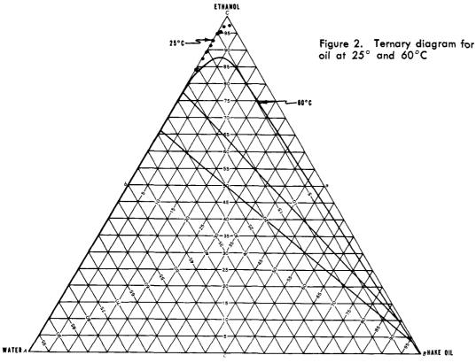
Figure 2. Ternary diagram for system water-ethanol-hake
